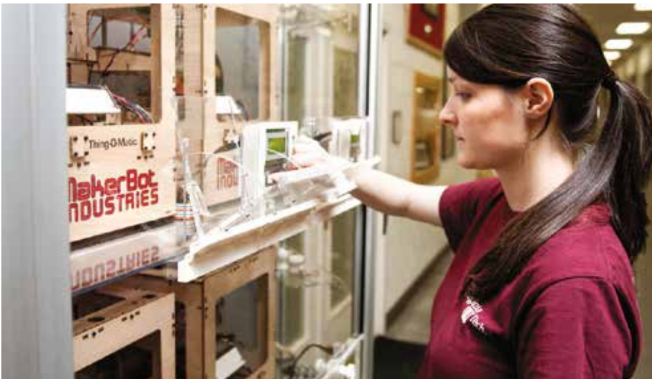
Similar to inserting coins to buy a snack, Virginia Polytechnic Institute and State University (Virginia Tech) students like Amy Elliot (above) insert an SD card with their design into DreamVendor, and the machine fabricates and dispenses a finished part. Amy is researching additive manufacturing of copper for her Ph.D. work in the Virginia Tech DREAMS Laboratory. (Photo courtesy of Virginia Tech.)
