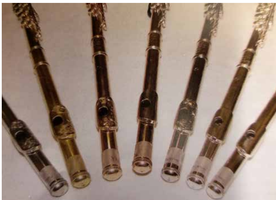
At the Institut für Wiener Klangstil (IWK) in Austria, researchers tested seven identical flutes made out of silver, various degrees of gold, and platinum, as well as coated instruments, to determine if the sound quality from the different flutes was affected by the choice of material. (Photo courtesy of the IWK)
