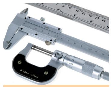
Measurements are only as accurate as the device used since the instrument determines how many significant figures you can obtain. A standard ruler cannot be read beyond 2 or 3 significant figures, but a micrometer might allow you to provide a more detailed measurement.
