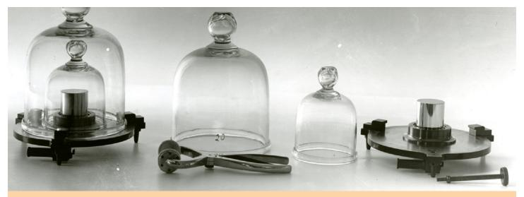
The International prototype kilogram was once the primary standard kilogram for the entire scientific community but was replaced in 2019 with a new definition based on constants occurring in nature. (Photo courtesy of The National Institute of Standards.)
