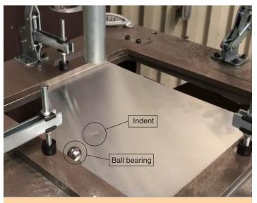
The experiment you are conducting is similar to how scientists test the extent to which car hoods can withstand hail damage. A large ball bearing is dropped onto a sheet of metal and the indentation is then measured and recorded. (Photo courtesy of Arconic.)
