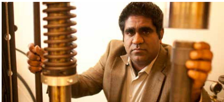
A materials scientist and avid comic fan, Suveen Mathaudhu has the “super power” of being able to modify the microstructure of metals by using advanced scientific tools and techniques. In this photo, he is shown performing a compression test on a Dake 70-ton uniaxial load press, pushing a metal sample until it fails and recording the load and displacement along the way. This helps him determine how a material will perform in a real-world application.
